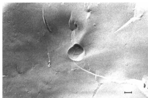
FIGURE 8 Freeze fracture electron micrograph of 4k vesicular solution. Bar length is 100 nm.
